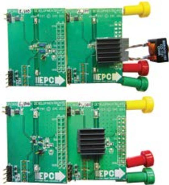
Figure 4: Experimental boards showing standard and modified EPC9002/6 development boards.
